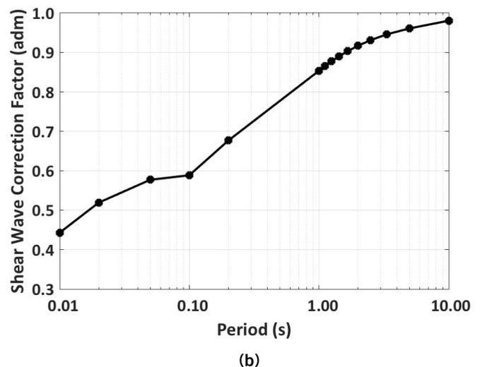
Fig. 3 - Rock to hard rock corrections for TST site at Euroseistest. (a) Crustal amplification functions for a standard rock site ( $V_s=800$  m/s, blue) and for a hard-rock site ( $V_s=2,600$  m/s, green). (b) The Shear Wave Velocity Correction (VSC) corresponding to the ratio between these two quarter-wavelength crustal amplification functions.
