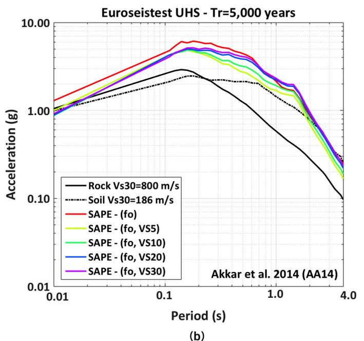
Fig. 12 - (a) Site amplification factors estimated at TST<sub>0</sub> station from site amplification prediction equations (SAPEs, Cadet et al., 2012b) with different proxies; (b) Corresponding 5000 years UHS using Akkar et al., 2014 GMPE and the various SAPEs.
