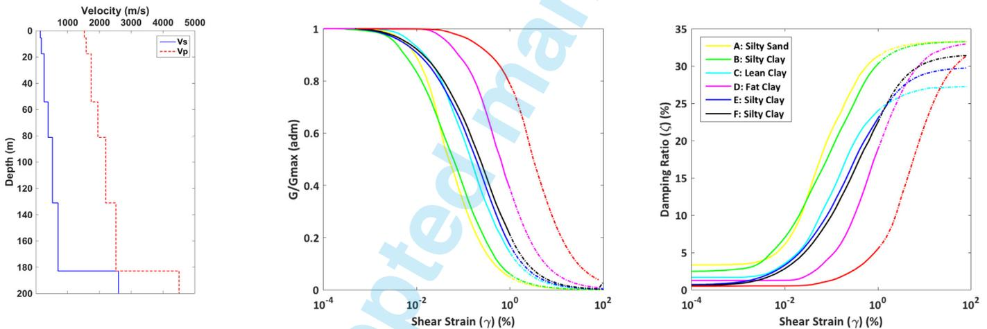
Fig. 2 - Euroseistest case study: (a) 1D shear wave,  $V_s$ , and compressive wave,  $V_p$ , soil profiles between  $TST_0$  and  $TST_{196}$  stations (see Figure 1b) based on Raptakis et al., 1998; (b) non-linear degradation curves showing the decrease of the shear modulus with shear strain, and (c) the increase of shear damping with shear strain (Pitilakis et al., 1999).
