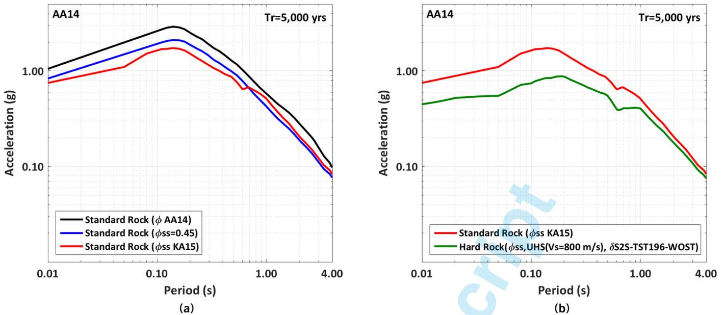
Fig. 8 : Euroseistest site, TST site, UHS at 5000 years return period: (a) Calculation for standard outcropping rock at TST site, impact of the single-station within-event variability ( $\phi_{ss}$ ) on the UHS for three different values of  $\phi_{ss}$ ; (b) Scaling of the UHS on standard outcropping rock (red) by applying the site term ( $\delta S2S$ ), using  $\phi_{ss KA15}$  to obtain the UHS on hard rock at depth (green, TST<sub>196</sub> station).
