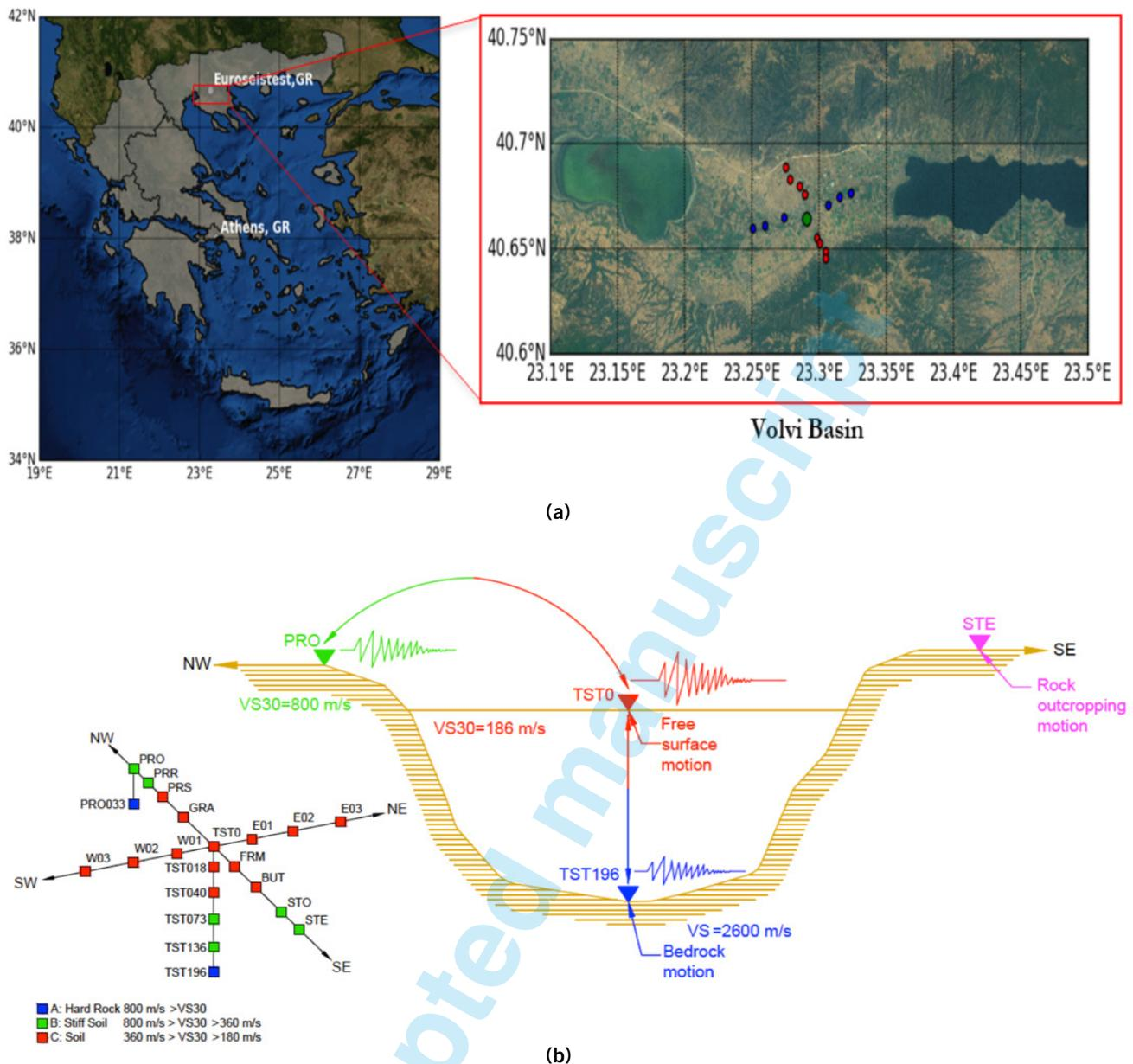
Fig. 1 - (a) Euroseistest location at Volvi basin in North Eastern Greece. (b) Euroseistest PRO-STE simplified cross-section with the main stations used in this study ( $TST_0$  and  $TST_{196}$ ), as well as the sketch of the current station array (modified from Pitolakis et al., 1999).
